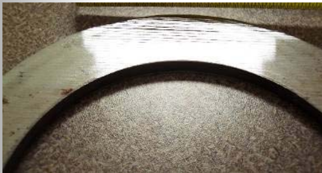
Tantalum on I.D. of steel pipe
