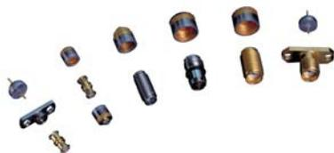
PA&E's 50 Ohm hermetic RF/Microwave connectors are designed for use in military and commercial applications where environmental conditions require an extremely rugged and reliable hermetic seal. Low-loss Corning 7070 glass is used for dependable electrical performance. PA&E manufactures these hermetic RF connectors from a variety of compatible shell and contact materials, in both laser weld and solder-in styles, which provide excellent electrical and environmental performance characteristics.
