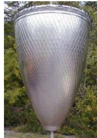
Space Shuttle Cone and After Explosive Forming
